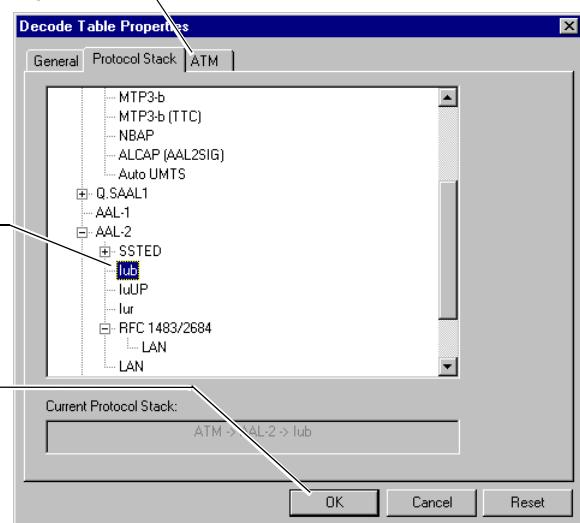
④ Edit the Defaults entry in the Decode Table to change the Protocol Stack to AAL-2 -> Iub.
