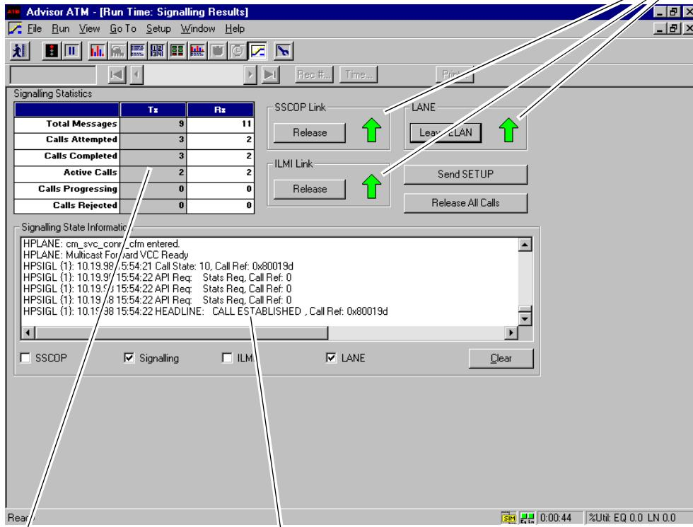
Statistics related to the calls made are shown in this spreadsheet. Notice that 3 calls originating from the Advisor (Tx - transmit) were successfully made. Also notice that 2 SVCs are currently active on each side of the test connection, showing that SVCs to and from the LAN Emulation Server (LES) and the Broadcast and Unknown Server (BUS) are active. This indicates that the emulated LAN was joined successfully.
