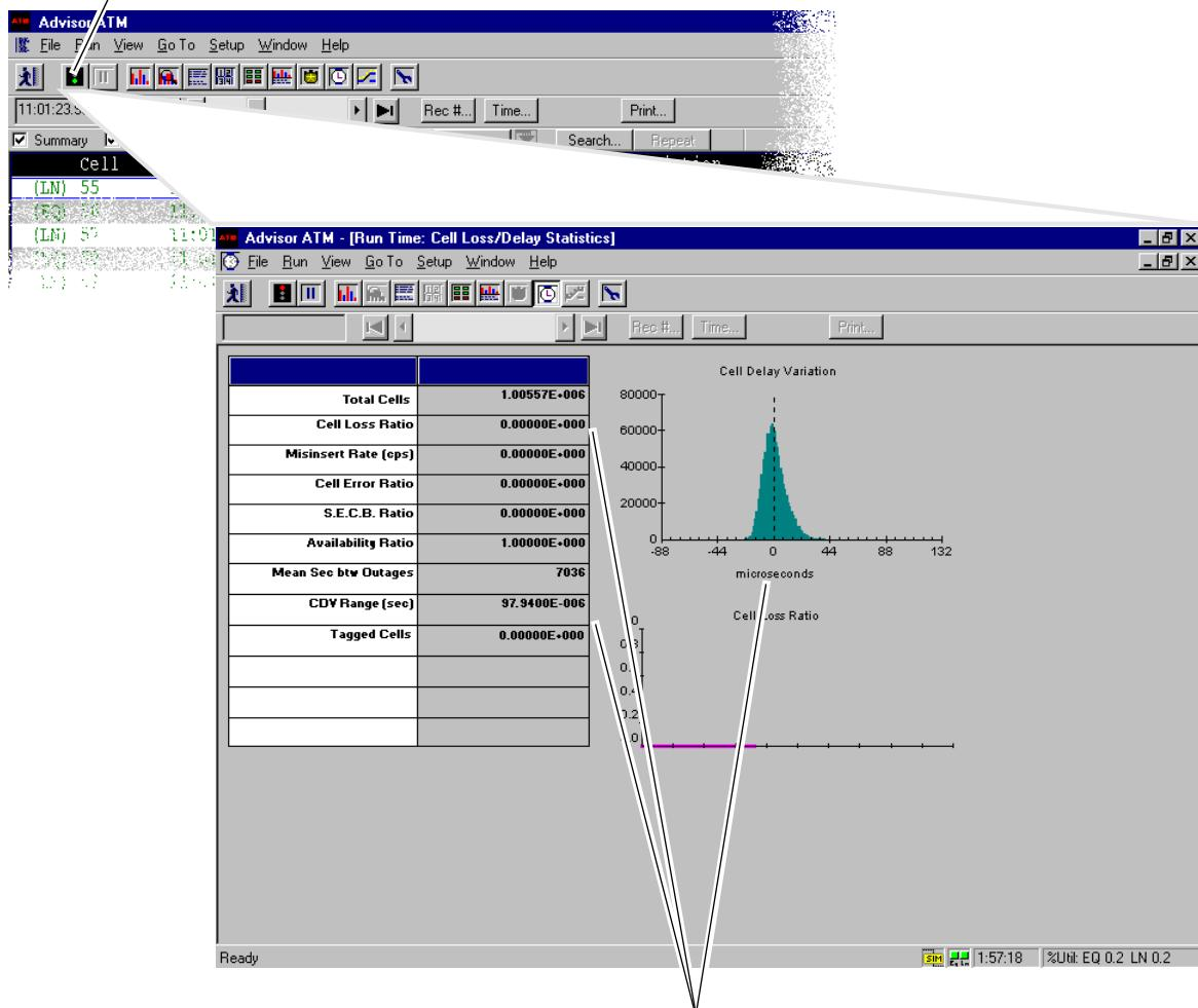
The Cell Loss/Delay Statistics view shows the results of measurements made on the incoming test cell stream. As you can see in this example, no cell loss is occurring, there is a Cell Delay Variation (CDV) range of 97.9 microseconds (acceptable in most cases), and no cells are being tagged. This indicates that the transmission path from the remote Advisor to this one is providing the QoS that you expect.
