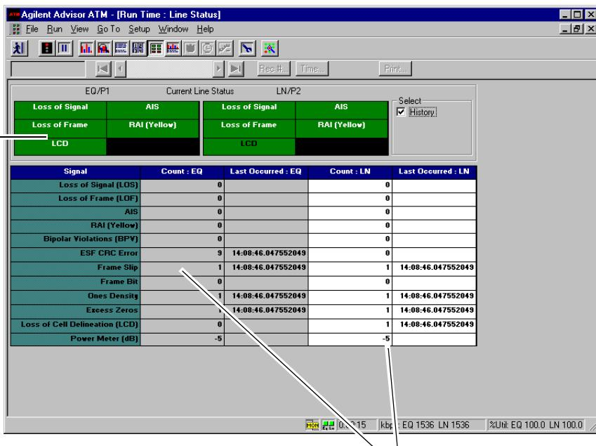
Use the on-screen 'soft' LEDs to see the status of physical layer transmission.
