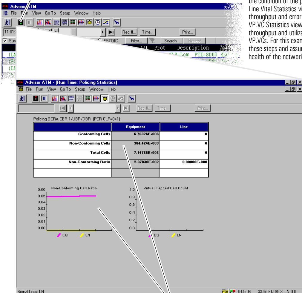
Note: in many troubleshooting scenarios you would often use other measurement views to verify basic network operation. For example, the Line Status view tells you the condition of the physical layer. The Line Vital Statistics view shows general throughput and error statistics. The VP.VC Statistics view shows you throughput and utilization for individual VP.VCs. For this example, we will skip these steps and assume the general health of the network is good.
