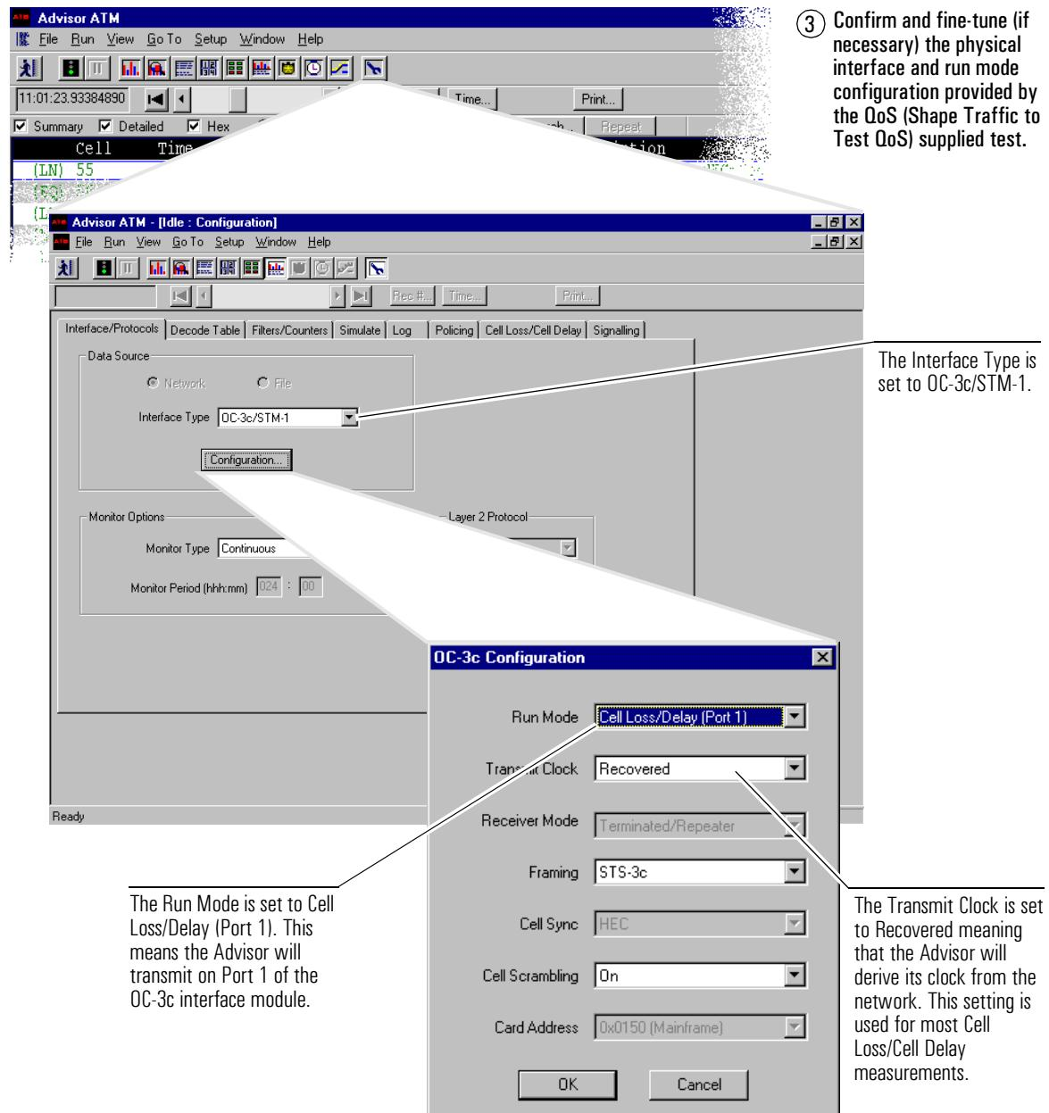
④ Bring the Cell Loss/Cell Delay folder to the front so you can configure measurement-specific parameters.
