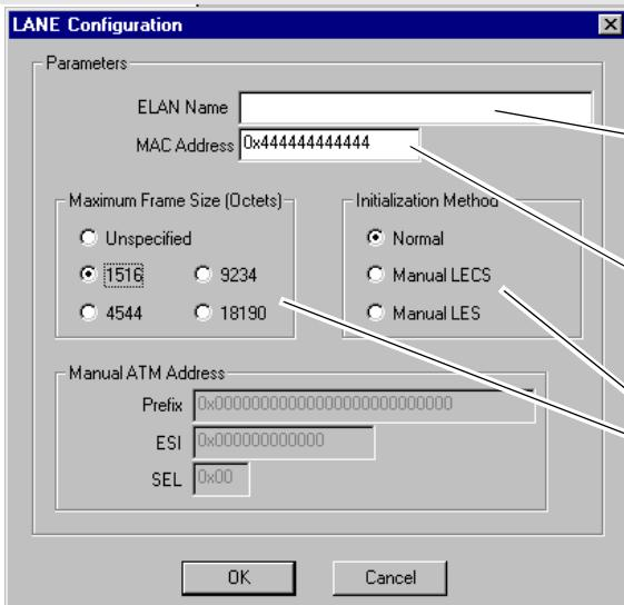
⑦ Type in the name of the emulated LAN you want to join. You can leave this box blank and the LANE configuration process will provide the name.
