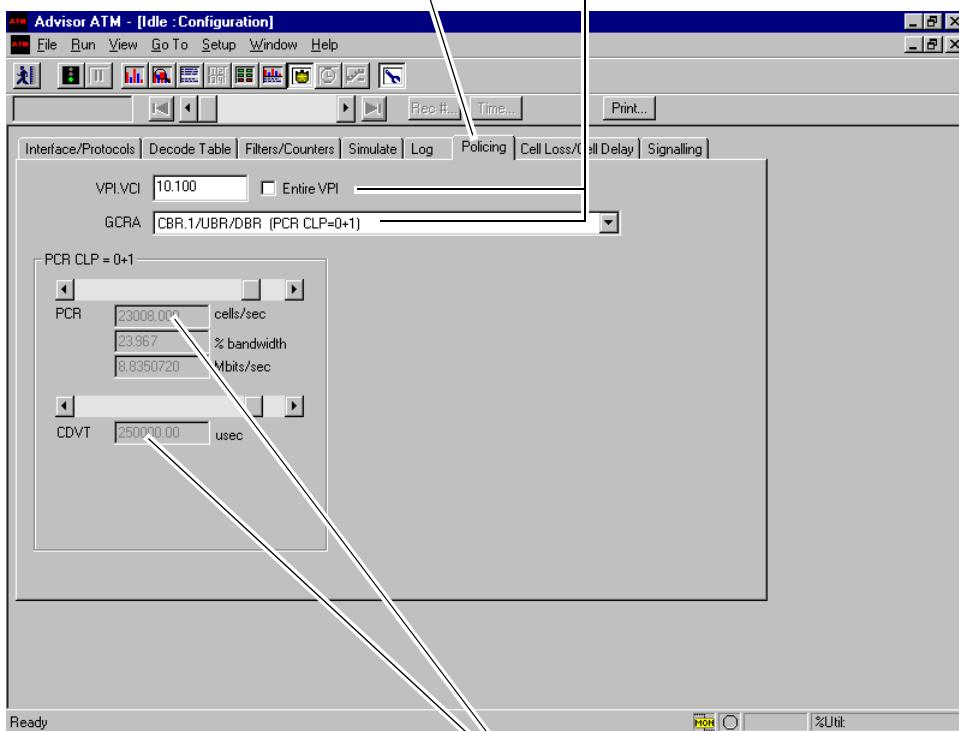
⑤ Select the VP.VCI you want to monitor and the Generic Cell Rate Algorithm (GCRA) used by the network you are testing.
