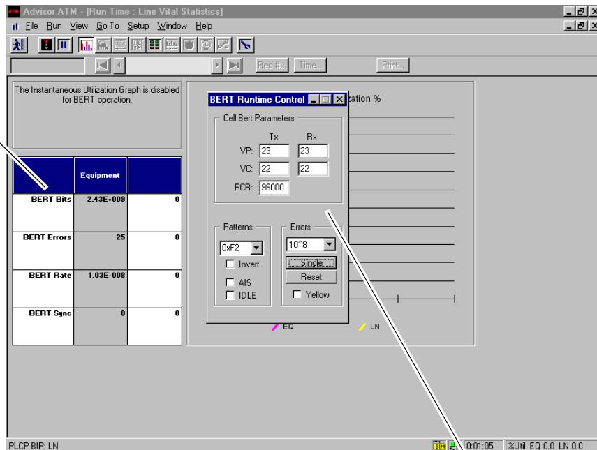
You can control the characteristics of the bit error rate test during runtime.
