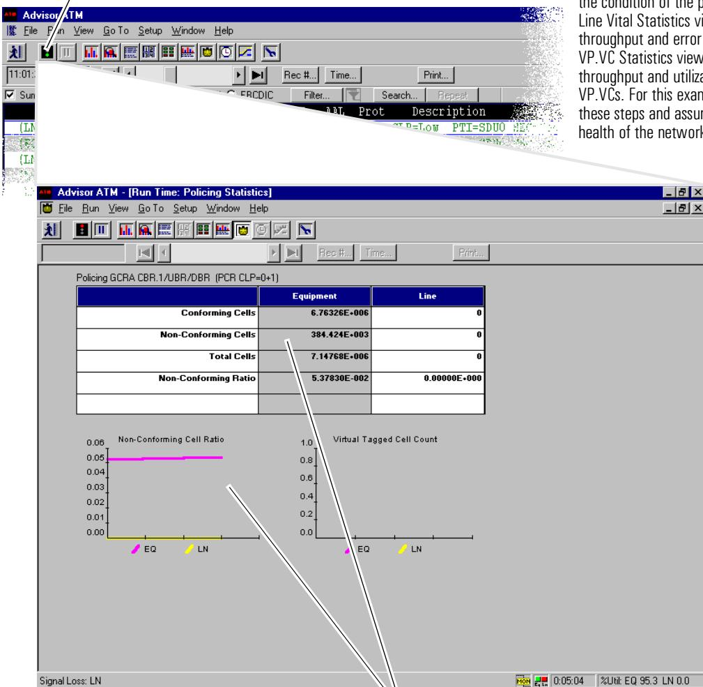
Note: in many troubleshooting scenarios you would often use other measurement views to verify basic network operation. For example, the Line Status view tells you the condition of the physical layer. The Line Vital Statistics view shows general throughput and error statistics. The VP.VC Statistics view shows you throughput and utilization for individual VP.VCs. For this example, we will skip these steps and assume the general health of the network is good.
