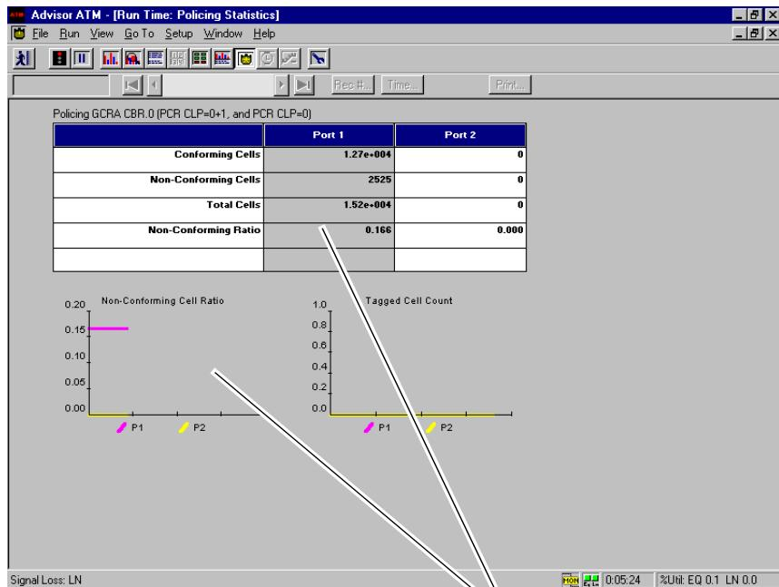
You can see how ATM traffic may be affected by the network's policing algorithms in a spreadsheet and in graphs.
