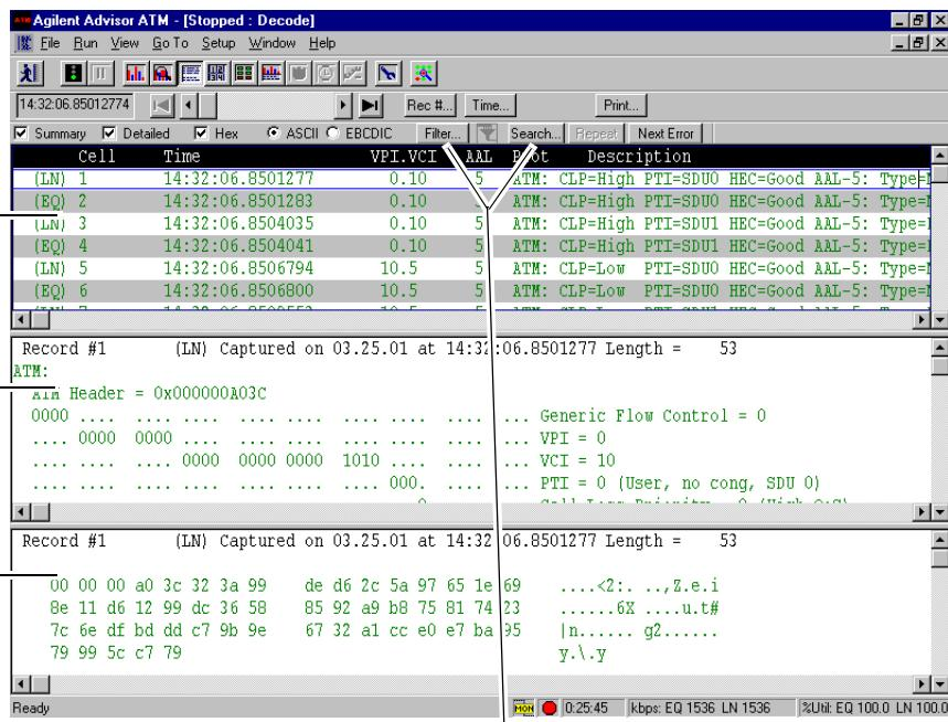
You can filter what is displayed in this view, and you can search the capture buffer for specific cells/PDUs or data events.
