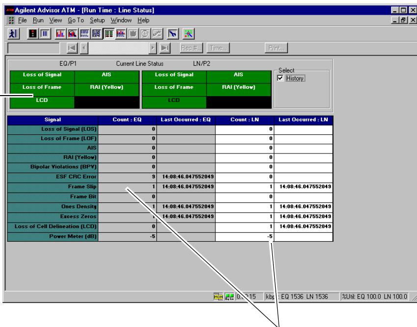
Use the on-screen 'soft' LEDs to see the status of physical layer transmission.
