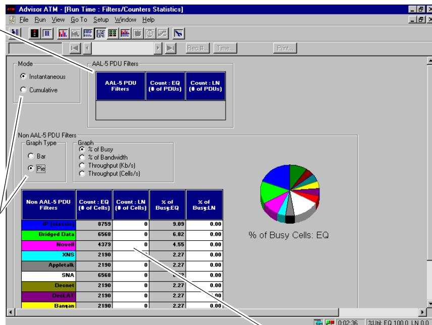
Filter and count traffic based on ATM cell characteristics.
