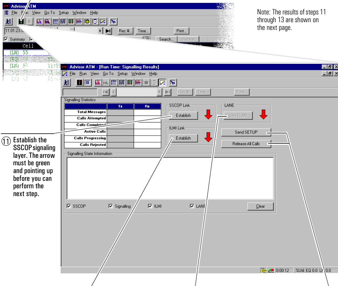
⑪ Establish the SS/CP signaling layer. The arrow must be green and pointing up before you can perform the next step.
