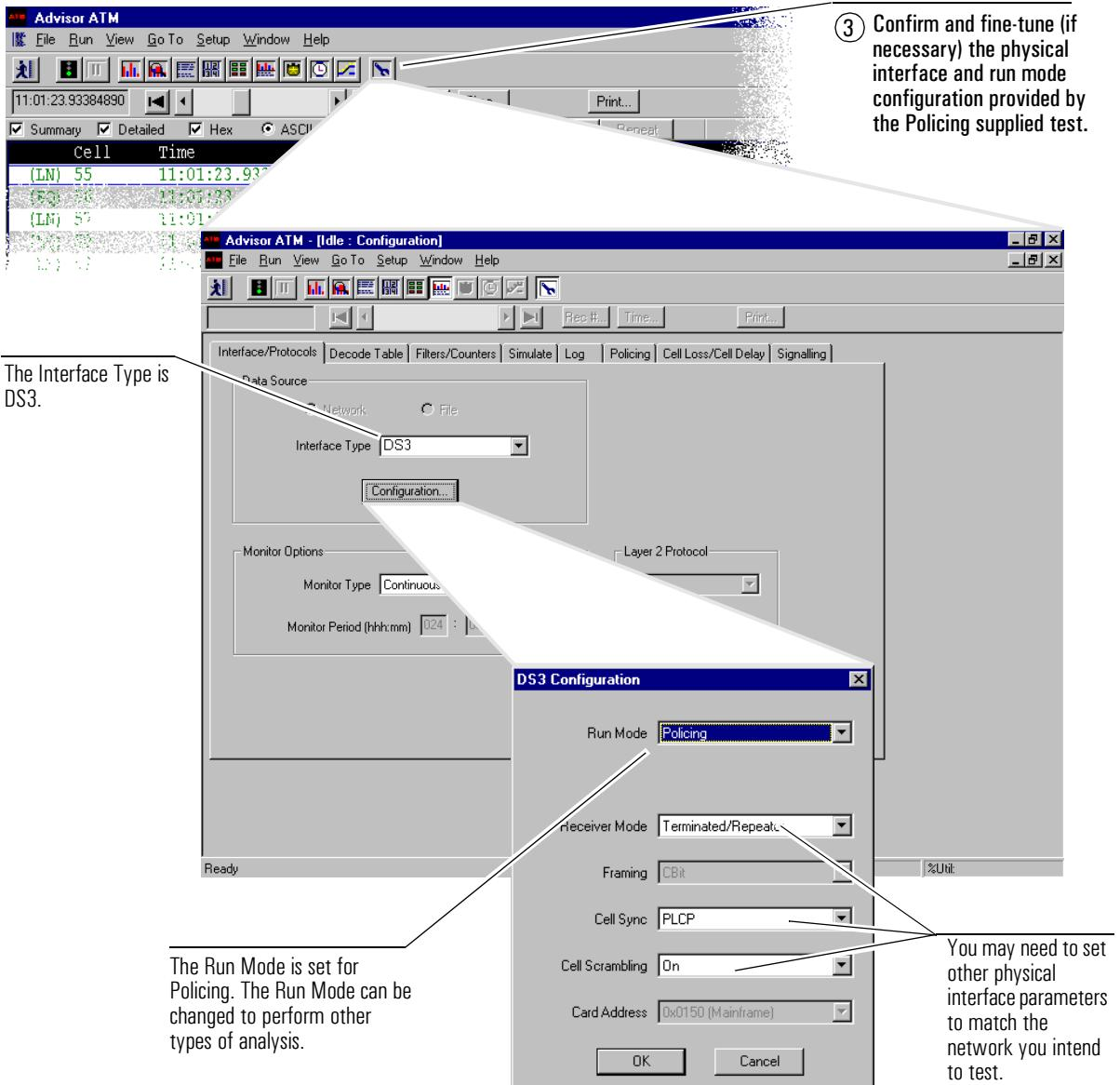
④ Bring the Policing folder to the front so you can configure measurement-specific parameters.
