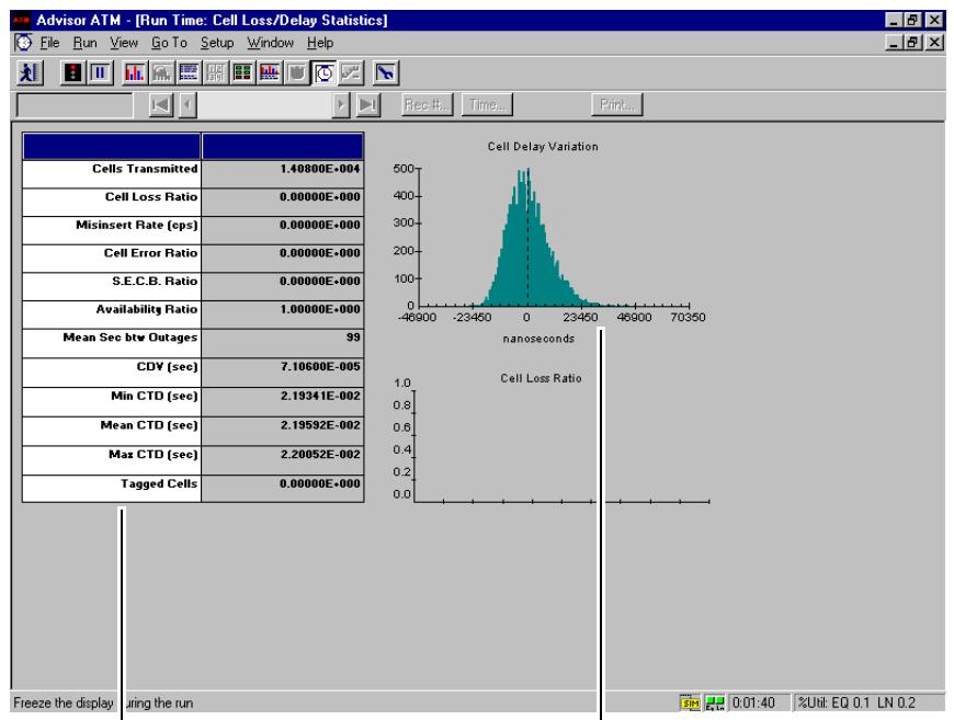
See the results of the cell loss and cell delay measurement in the spreadsheet.
