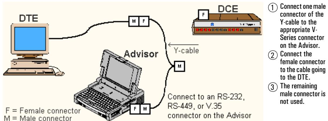
Caution: When using a Y-cable to attach the Advisor to a DTE, take care to keep the pins of the unused male connector from making contact with any metal object. This is especially true for the V.35 male connector. The signal levels are very low energy, and therefore not dangerous, but accidental short circuits can cause improper operation of the DTE and unreliable data collection by the Advisor.
