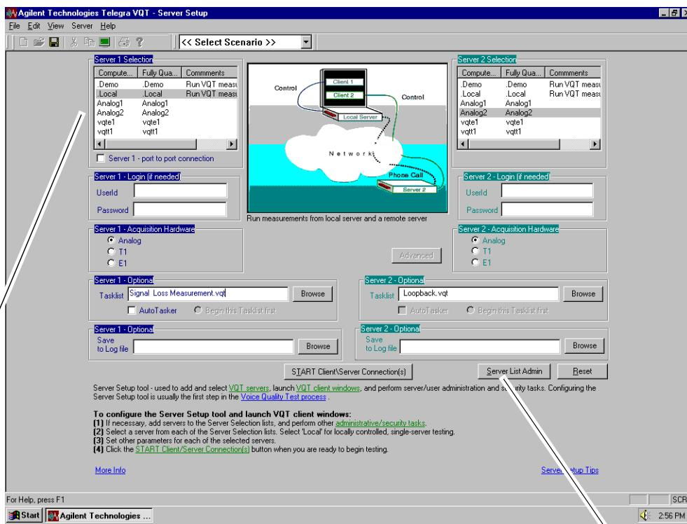
If you plan to perform locally controlled, single server testing, click "Local" in the Server Lists, click the Start Client/Server Connections button, and begin testing.
