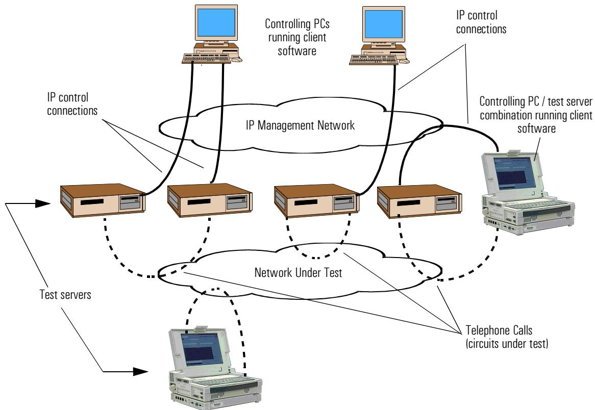
As shown above, the VQT system consists of “controlling PCs” (running “client” software) that operate “test servers”. The controlling PC and the test server can be the same device, and the test server can be one of several Agilent VQT devices including the VQT Portable Analyzer.
