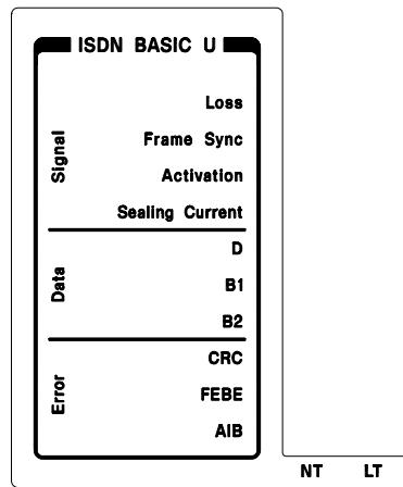
Loss - shows green if signal is present; red if no usable signal can be detected.
