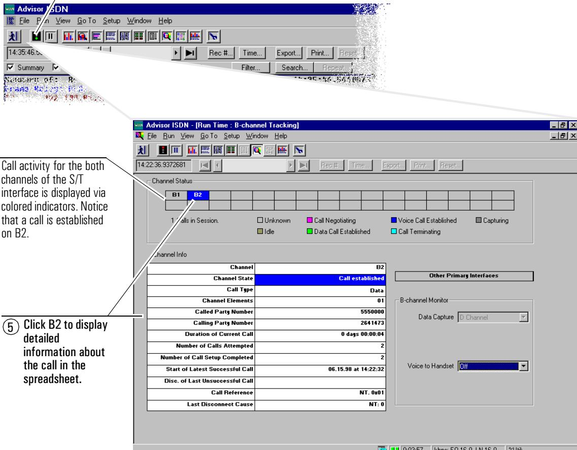
To understand why calls are unexpectedly disconnected, observe the call activity until a disconnect occurs. This is shown in the Channel Status indicators at the top of this measurement view. In this example, assume B2 disconnects abnormally (shown in next illustration).
