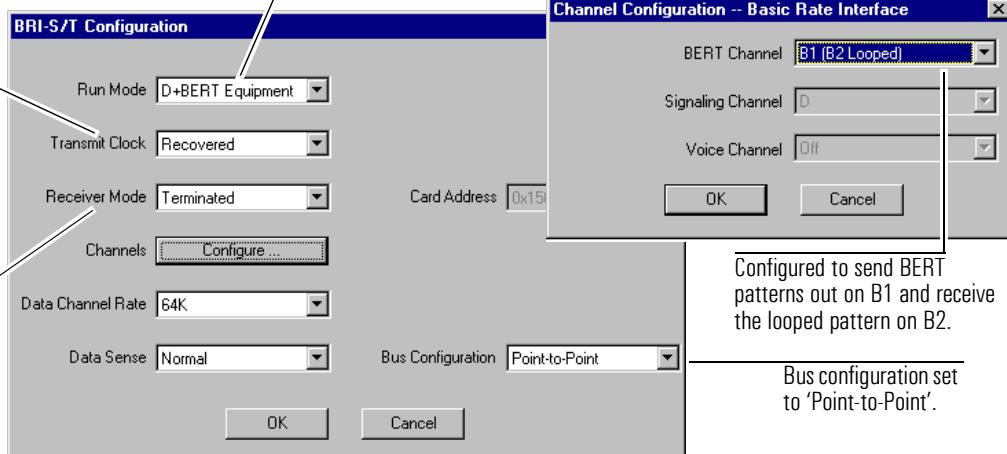
⑫ Set the parameters necessary to place and maintain the loopback call.
