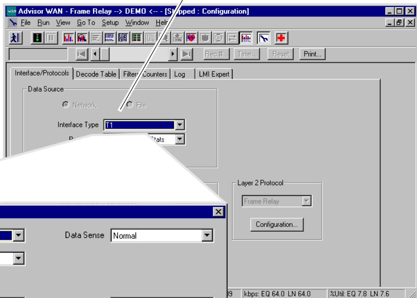
④ Set the Receiver Mode, Line Code, and Framing parameters.
