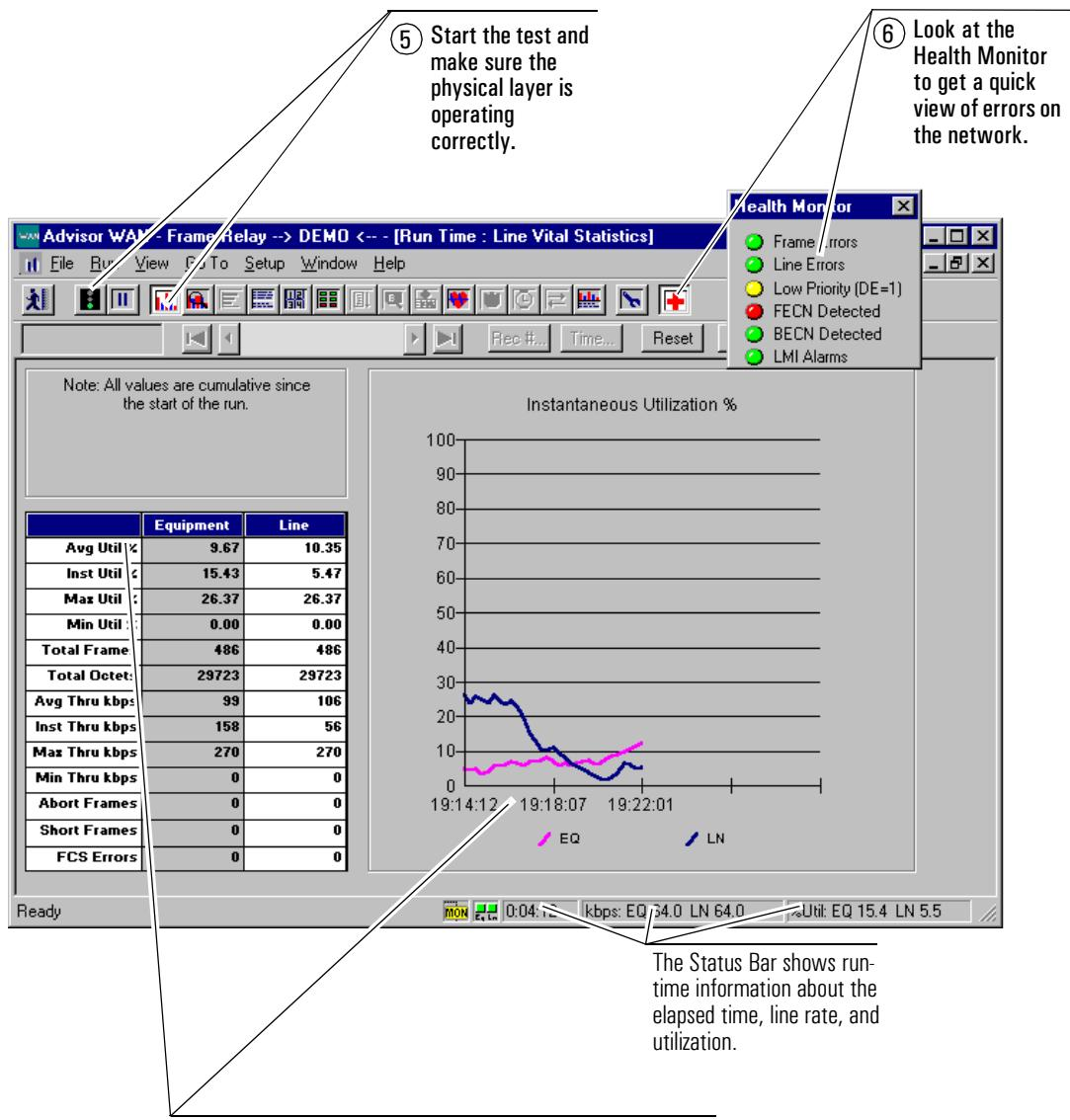
You can see the utilization, frame and octet counts, and throughput updated for both the Line and Equipment sides of the connection. The graph shows instantaneous utilization.
