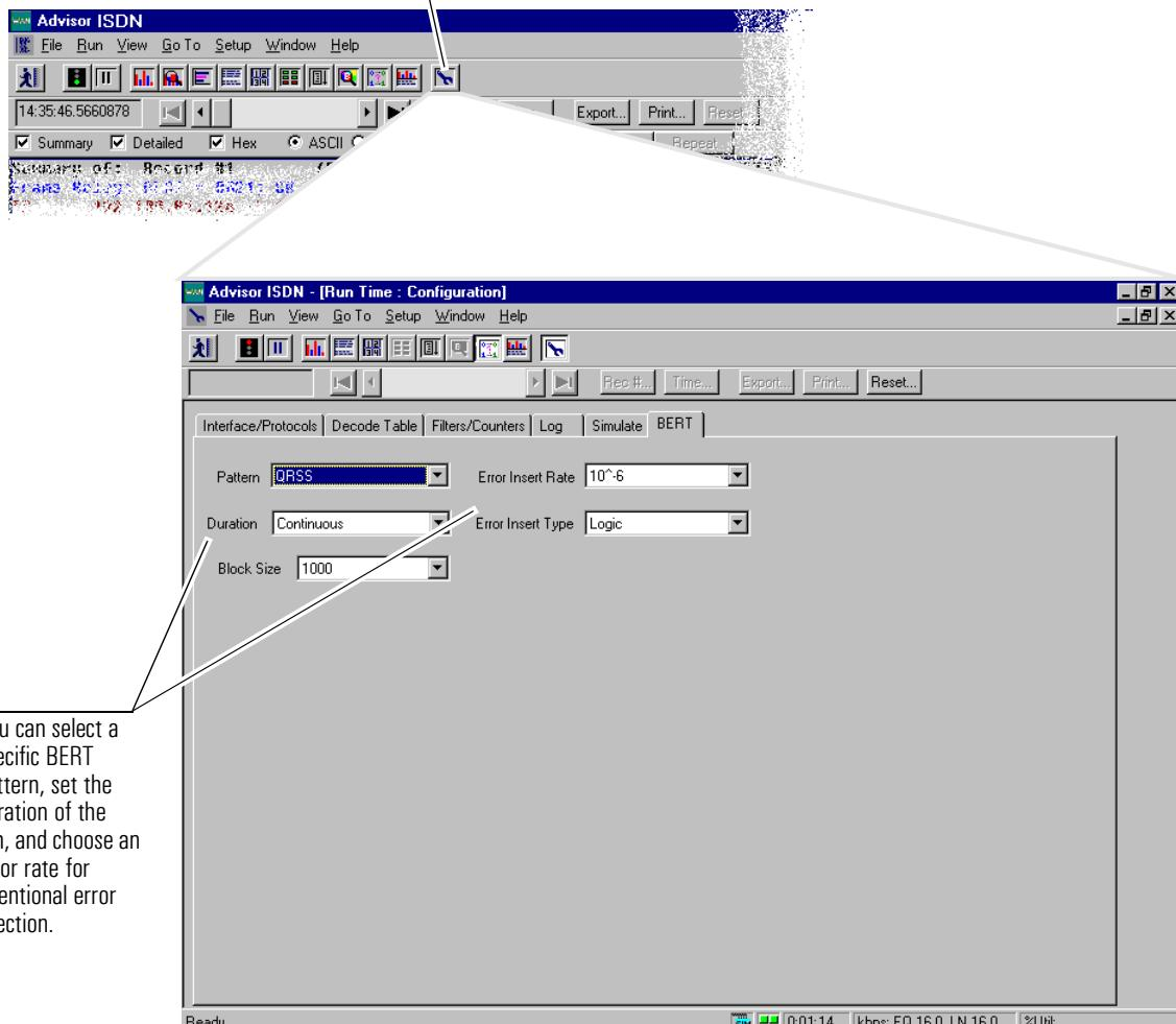
You can select a specific BERT pattern, set the duration of the run, and choose an error rate for intentional error injection.
