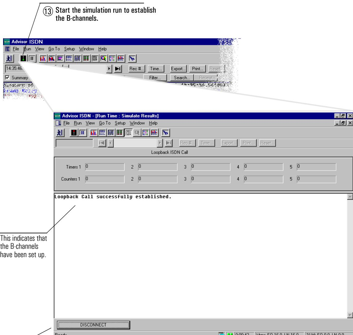
Note: when you start a simulation/BERT test, error messages may be displayed if you have not set all of the necessary simulation parameters. For example, if you have forgotten to define the Calling Number in the Simulate folder, or the BERT channel in the BRI S/T Configuration dialog box, an error message will be displayed and the simulation script will not execute.
