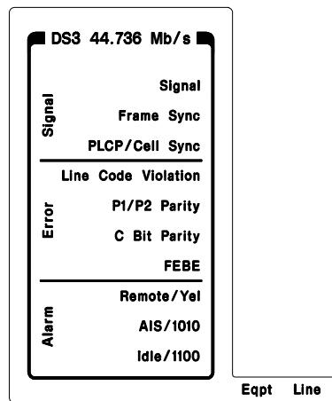
Signal - shows green if signal is detected, red if no signal detected.
