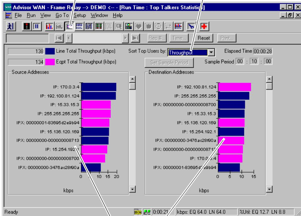
You can see which IP and IPX users are transmitting the most data, sorted according to source and destination. This view is updated and represents the average 'top talkers' in the current measurement period.
