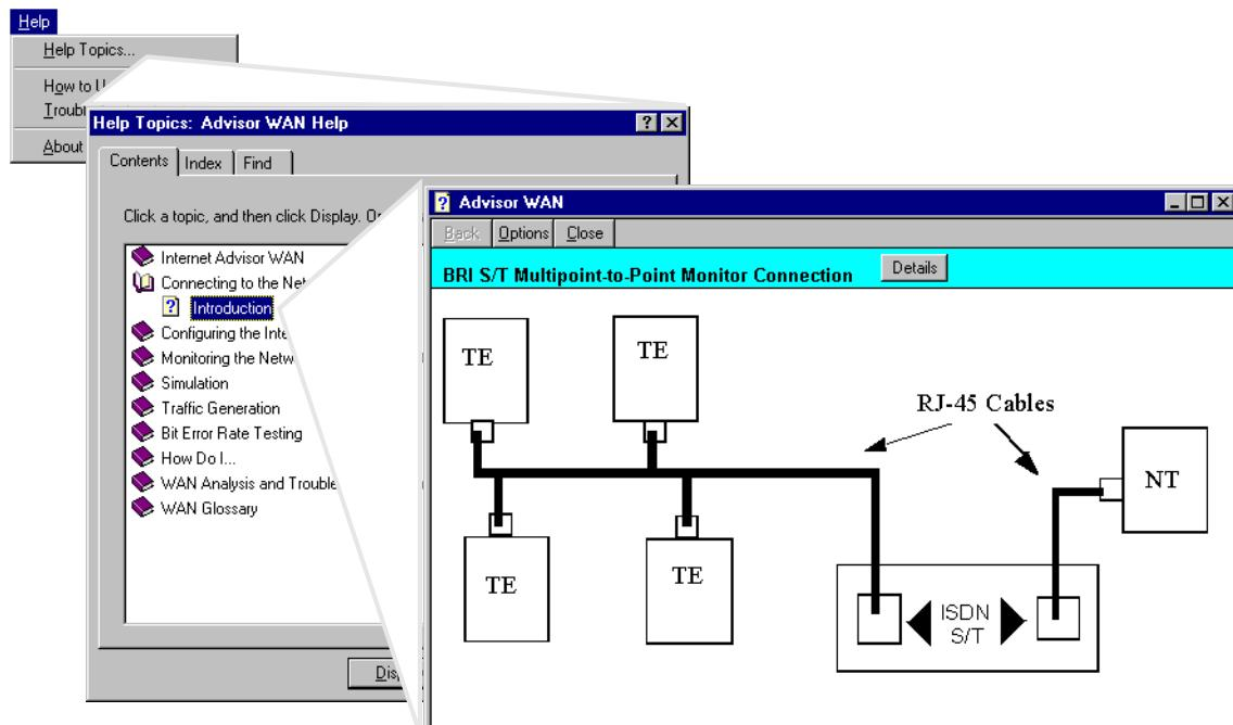
③ Confirm the configuration provided by the 'Analysis of ISDN Calls' supplied test.
