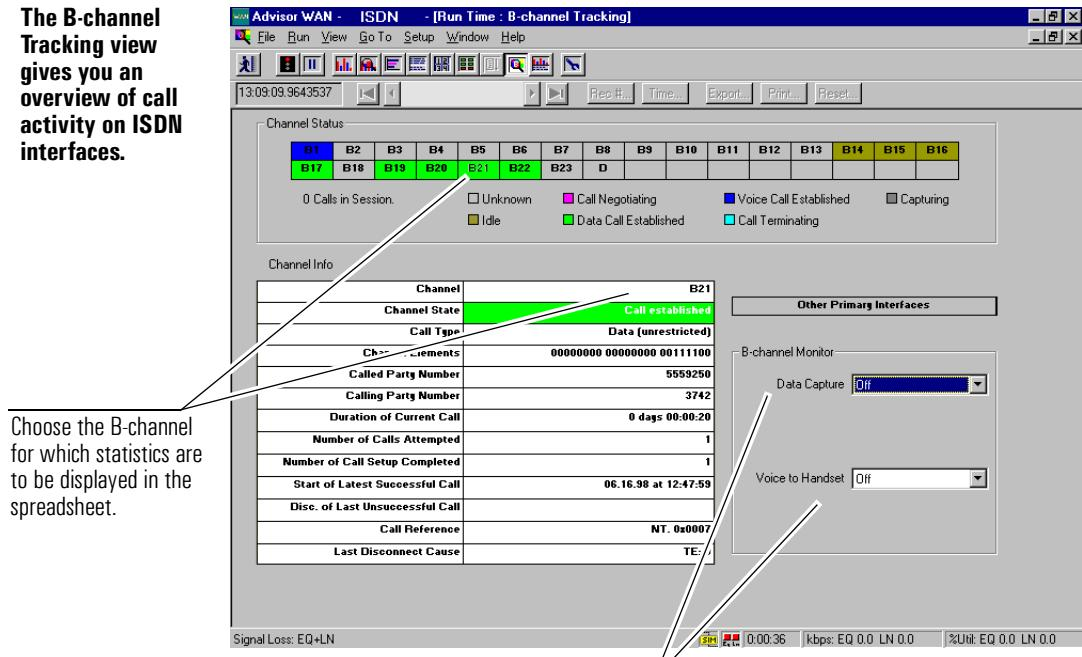
Control which B-channels are analyzed and how the data is to be captured.
