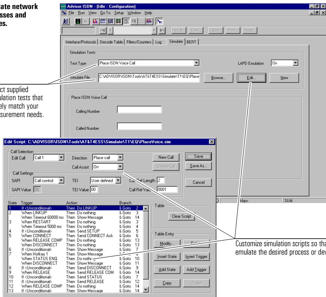
Customize simulation scripts so that they emulate the desired process or device.
