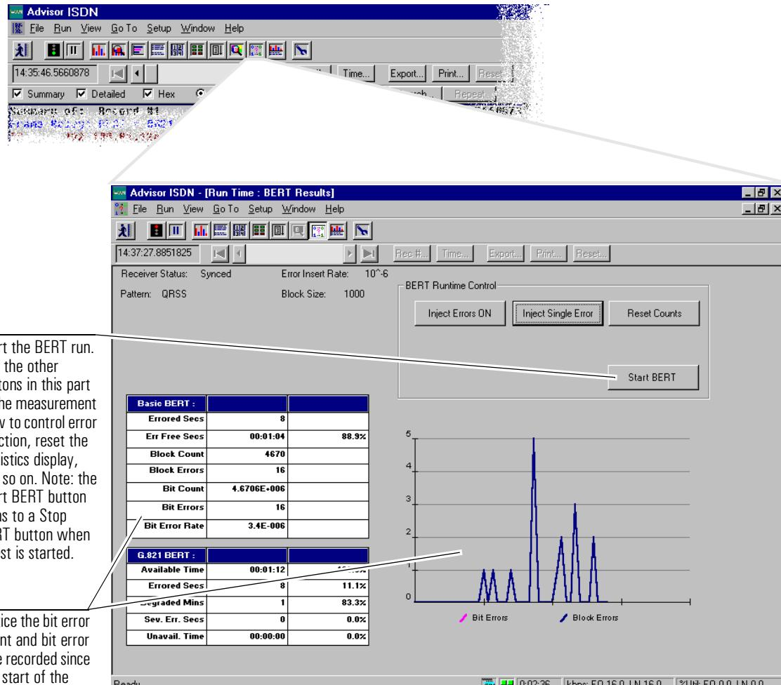
While this bit error rate is relatively low, it could be enough to garble layer 2 and 3 'keep alive' messages, resulting in calls being unexpectedly disconnected.
