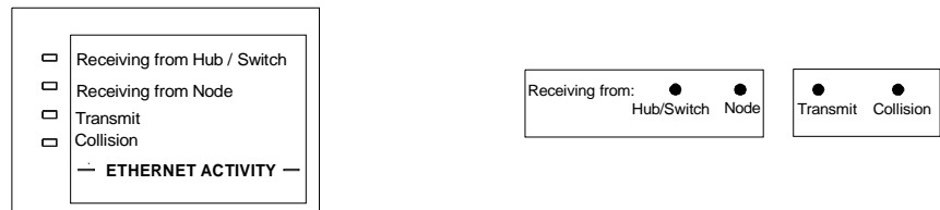
Figure 2-30: Ethernet Activity LEDs
