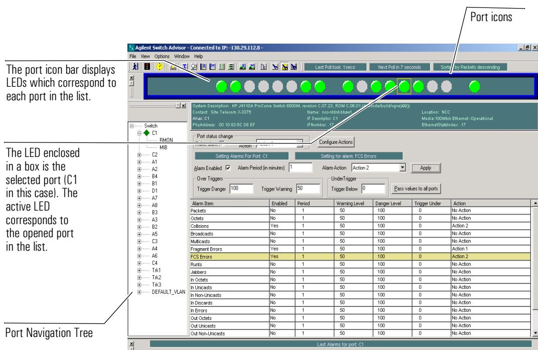
The port icon bar displays LEDs which correspond to each port in the list.
