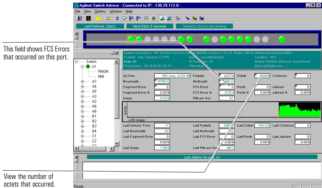
5 Select the Traffic Flow button. This view displays all ports showing LAN port usage and its associated percentage of utilization, along with number of packets that were Broadcast or Unicast.
