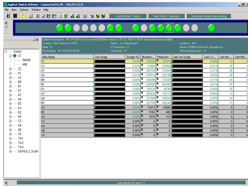
6 Select the Port Usage button. This view graphically displays the utilization level on each port.
