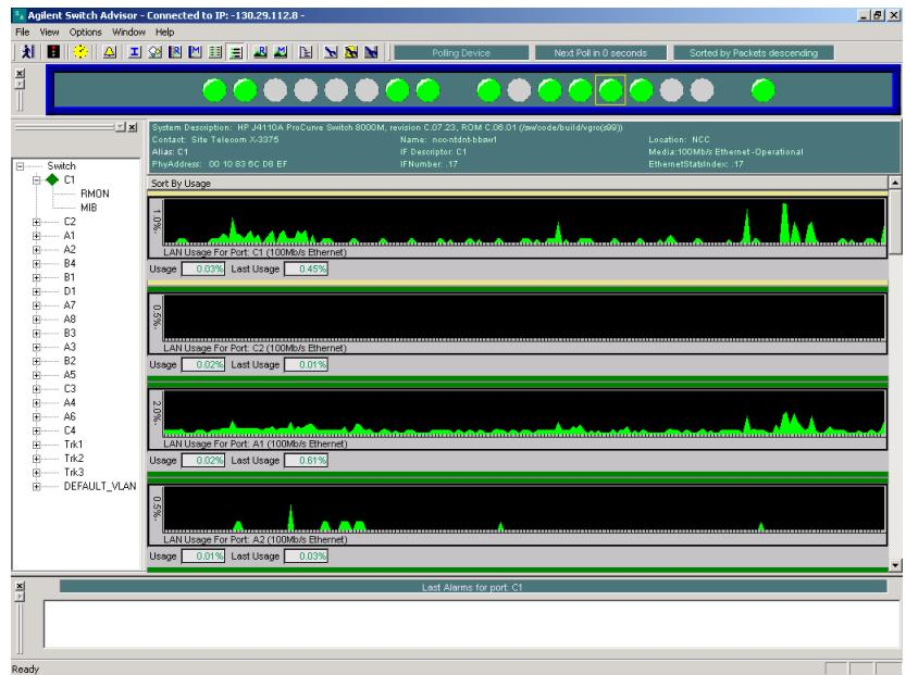
The sorting of Packets in descending order is maintained, so you visually see the utilization level of each port in the device under test.
