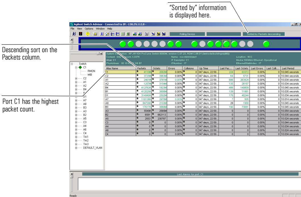
In this example, port C1 has the highest packet count. This is a quick way to see which ports of the selected device are the top talkers.
