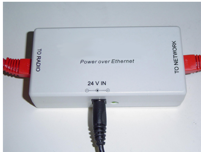
Figure 2-11: Power-Over-Ethernet (POE) Injector
