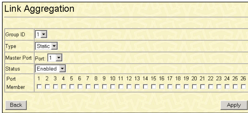
Figure B-23: 2 nd Link Aggregation window
